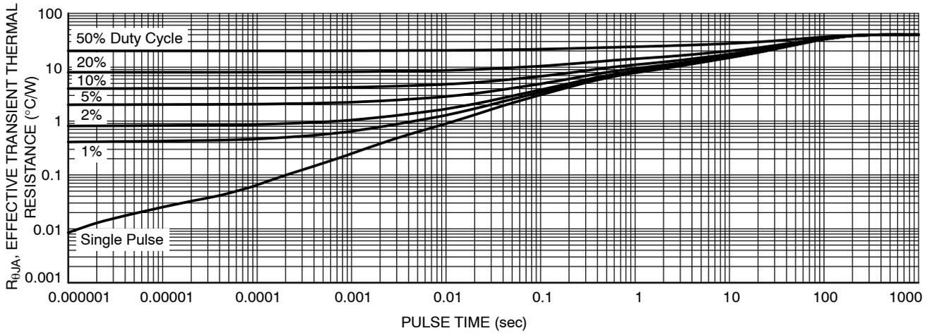
Figure 13. Thermal Characteristics
