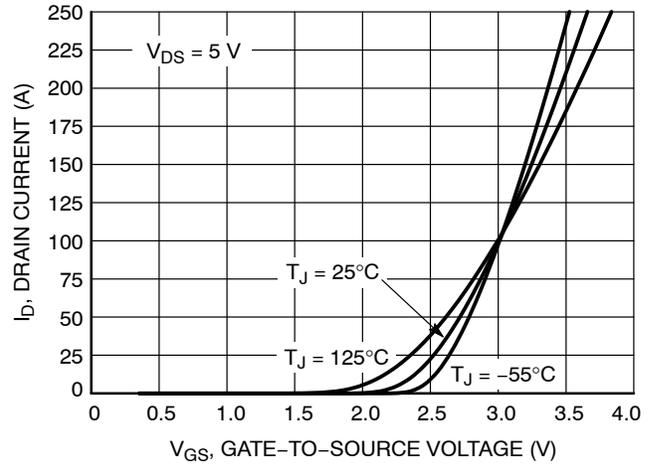
Figure 2. Transfer Characteristics
