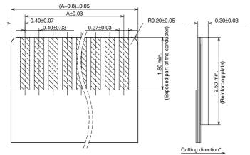
\*Cut FPC from the copper foil side to the reinforcing plate side.
